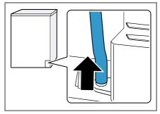
The condensation hose is connected to the connecting piece at the factory.
