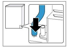
**3.** Push the water outlet hose as far as it will go into the connecting piece.
