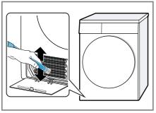
Ensure that you vacuum the fins from top to bottom so that they do not become deformed or damaged. 4. Clean the opening with a soft, damp cloth.
