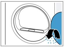
3. Remove the two-part fluff filter.
