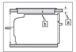
The minimum worktop thickness **b** a is based on the required minimum clearance **a**.
